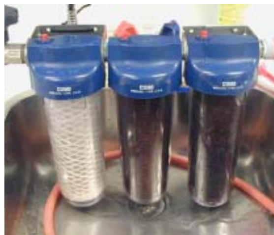
Figure 36. Pre-concentration of ^{137}\text{Cs} from seawater on hexacyanoferrate impregnated cartridges prior to gamma analysis.
