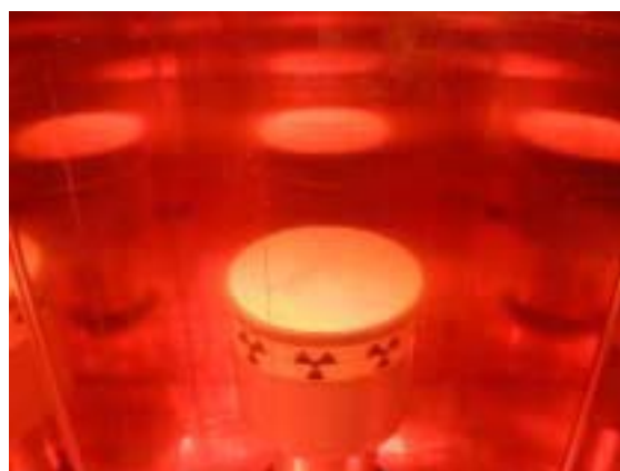
Figure 35. Analysis of a sample on a high resolution gamma ray spectrometer.
