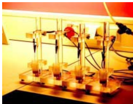
Figure 38. Electroplating of ^{99}\text{Tc} samples.
