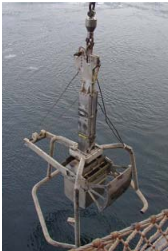
Figure 34. Sediment box corer.
