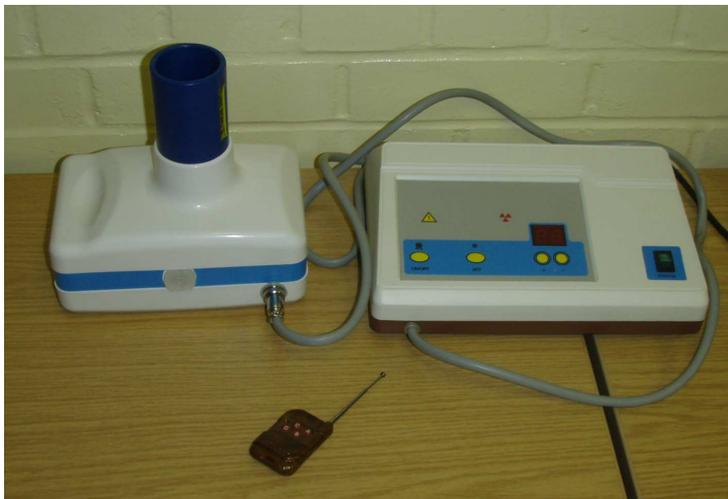
The operating potential and tube current are fixed and exposure times are selected on the control panel. Times can be selected between 0.1 and 9.9 seconds, in 0.1 second increments. X-ray exposures are triggered by either pressing an exposure button on the control panel or on the X-ray tube, or by using the remote exposure switch. The X-ray tube can be attached to a tripod if required but is intended to be used held in the hands.
