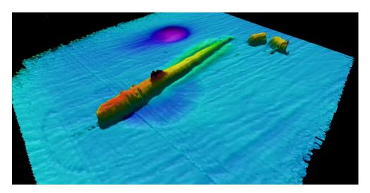
Figure 2.1 Acoustic model: a general view of the submarine on the sea bottom; two damaged pontoons are visible on the right.
