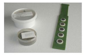
*Figure A.2.* Dried sample material in different containers ready for gamma measurements. To the right, <sup>99</sup>Tc preparations ready for counting.
