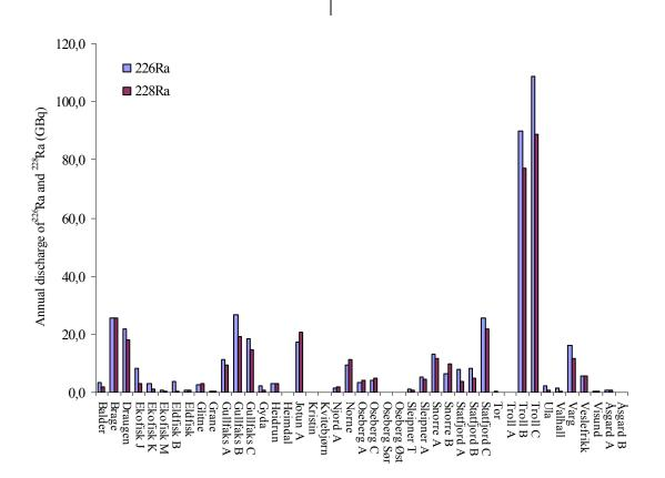
Figure 2.1. Estimated discharged activity of <sup>226</sup>Ra and <sup>228</sup>Ra from Norwegian oil and gas fields in 2006 (OLF, 2007).
