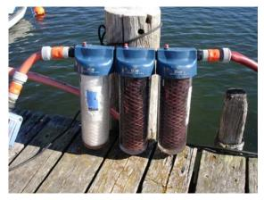
*Figure 3.3. Filter system used for analysis of* <sup>137</sup>*Cs in seawater.(Photo: NRPA).*
