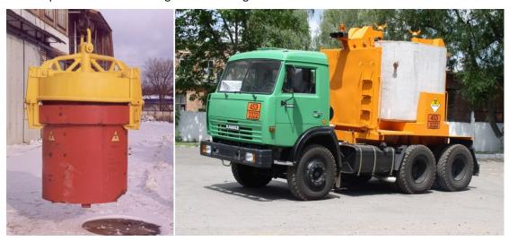
Fig. 4.4 Equipment for radioactive material transport
