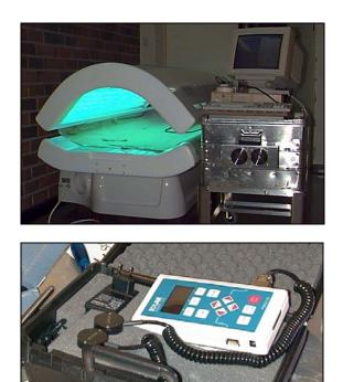
The spectroradiometer and the broadband radiometer with UVA and UVB sensors used during the inspection surveys.
