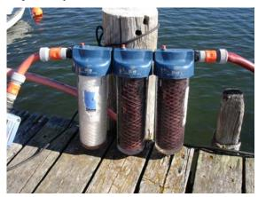
**Figure 3.3.** Filter system used for analysis of <sup>137</sup>Cs in seawater.(Photo: NRPA).
