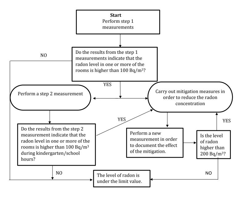
**Figure 1:** Flow chart illustrating the principals for measuring radon in schools and kindergartens
