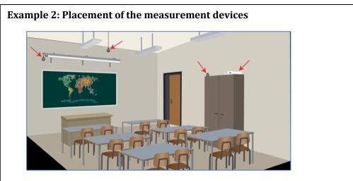
Measurement devices can be placed on the teachers' desk. Alternatively etched track detectors in step 1 measurements can be hung on a cord or placed on the top of a cupboard. On the top of a cupboard is also suitable for measurement devices in step 2 measurements.
