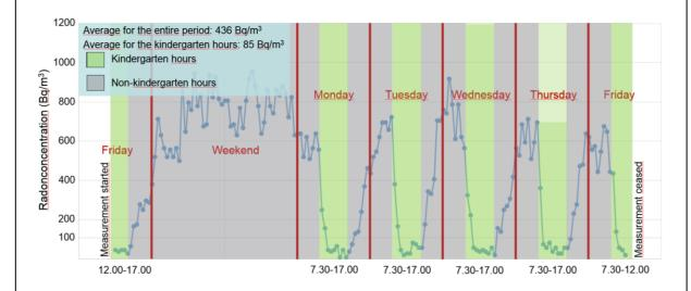
The follow up step 2 measurements showed that the radon concentration varied in the course of a twenty four hour period, depending on whether or not the ventilation was on. The average radon concentration for the entire measurement period was 436 Bq/m<sup>3</sup>. However during kindergarten hours the average was 85 Bq/m<sup>3</sup>.
