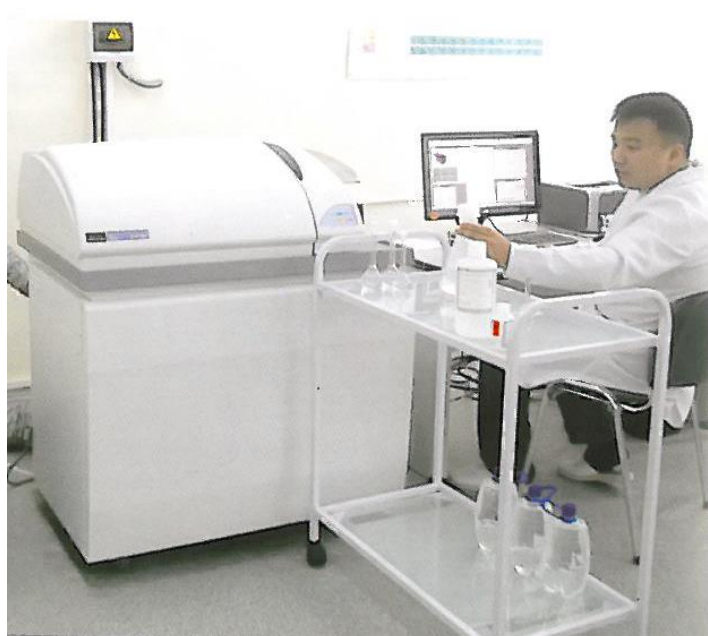
Left: Measurements of radioactivity in the human body. Right: the quadrupole mass spectrometer with inductively coupled plasma (ICP-MS) used for the measurements of radionuclides in environmental samples at RSE NNC in Kurchatov.
