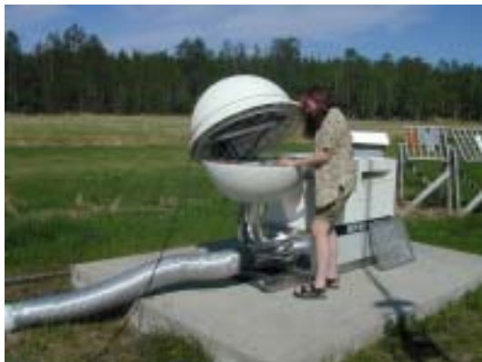
Changing of filters at the suction pump at Svanhovd. Photo: NRPA
