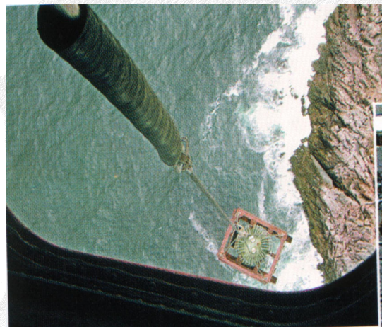
An RTG under helicopter transportation (Photo: Office of the County Governor of Finnmark)
