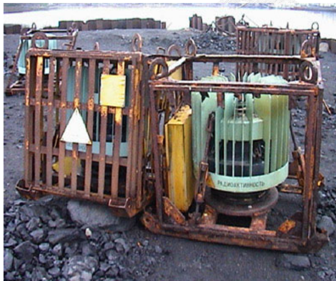
Retired RTGs awaiting decommissioning on the Kola Peninsula (Photo: Office of the County Governor of Finnmark).
