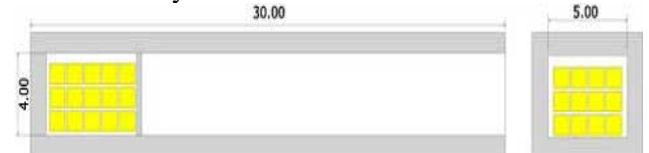
Sketch of a repository tunnel with concrete mould castings; units are measured in metres.
