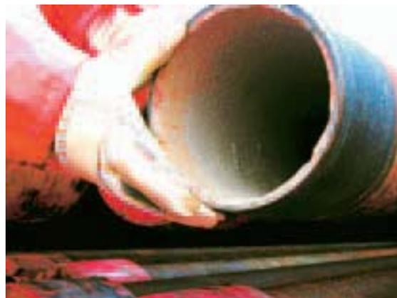
Figure 3.2. Hard scale deposits about one cm thick inside a production pipe. (Photo: Norwegian Radiation Protection Authority).
