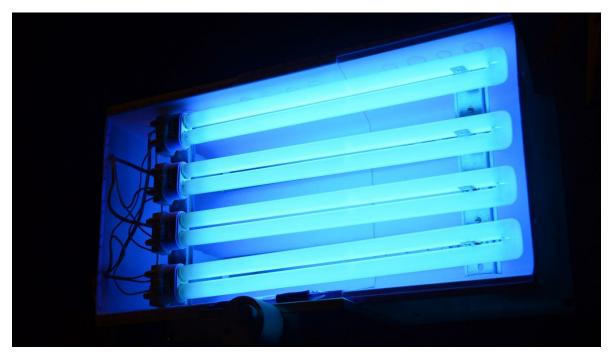
UVC tubes for sterilizing air and surfaces. Photo: Bjorn Johnsen, DSA.
