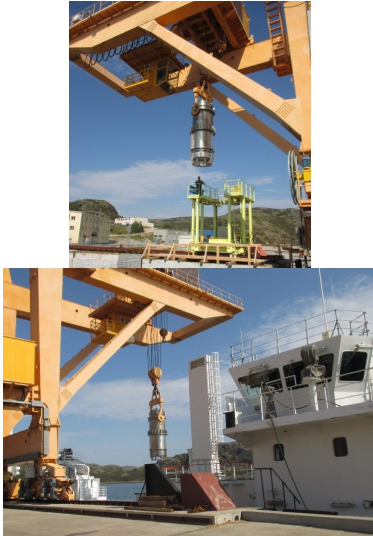
Figure 8. Process operations of loading the TUK-18 cask onto the container ship.
